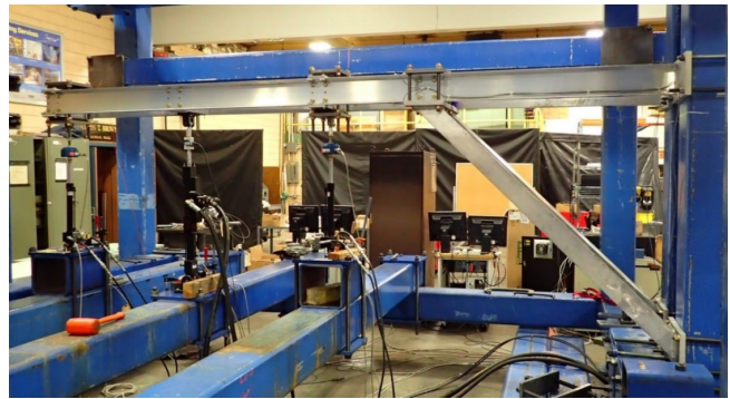
Figure 3 - Photograph of three actuator cantilever beam test setup used to investigated component IAC and PID load control systems.
