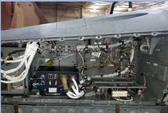
F-5N DADC/ADS-B modification/installation
