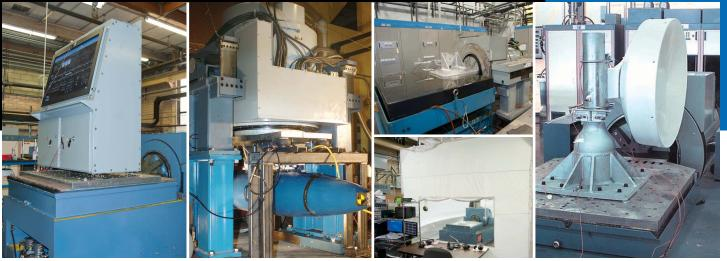
Our T5500-3 teamed with the T4000, T2000 and T1000 electrodynamic vibration systems further expand our vibration and shock testing capabilities. As the only independent testing lab that has a T5500-3, we provide higher force and displacement levels, compared to the traditional machines, saving you time, money, and meeting your requirements faster. Some of these upgrades include:
