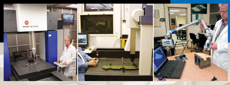
In DTB's Dimensional Lab, our highly trained staff examines your products from a critical perspective. Dimensional Inspection assures product compliance with design specifications by assessing the geometric characteristics that can affect both the reliability and functionality of the part. Our facility provides the capability to non destructively inspect selected parts from a first article or production lot, to confirm conformance to drawing requirements.
