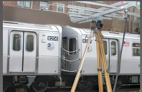
EMI/EMC On-site Testing
